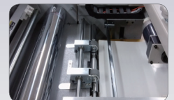
Photo 2) Automatic gap adjustment for feeding paper
